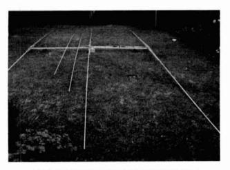
The complete triband beam prior to installation.
